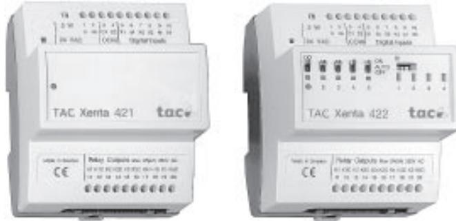
TAC Xenta 421 and 422 are Digital Input/Output modules in the TAC Xenta family. They are used as expansion modules for the TAC Xenta controllers and are connected by the common network.
