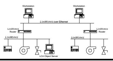
Figure 3. A fully distributed LONWORKS system using an Ethernet backbone
