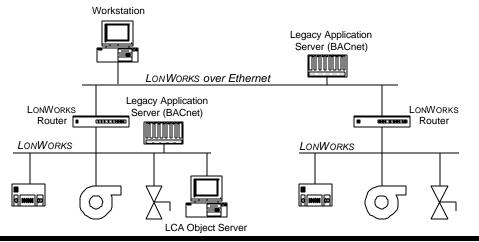
Figure 4. A fully distributed LONWORKS system with an Ethernet backbone using BACnet Servers
