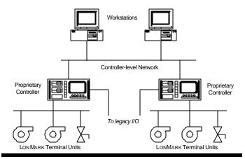
Figure 1. A typical system architecture today
