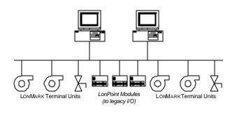
Figure 2. A fully distributed LONWORKS system
